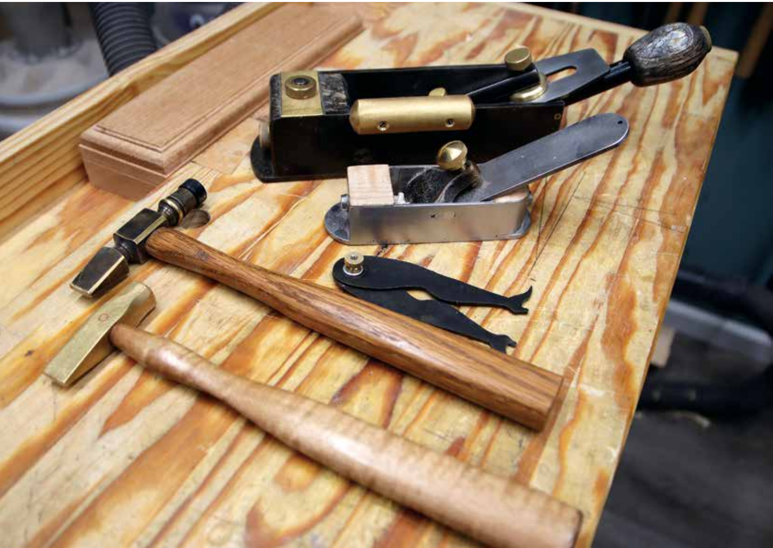
TOP: Meyer made these tools, including steel hand planes, a pair of Dancing Master calipers, and brass-head hammers. FAR LEFT: His space features assorted drills, clamps, and wood pieces. LEFT: To create a hand plane component, Meyer shaves down a hunk of curly maple. OPPOSITE: The decorative top of Meyer's Fish Head Hammer, used for plane setting, is made from a combination of 1095 and 15N20 steel.
